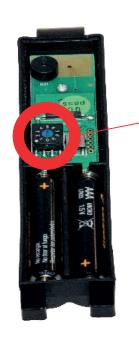
POUR RÉALISER LE PROGRAMMATION LE POTENTIOMÈTRE DOIT ÊTRE DANS LE POSITION " 0 "
